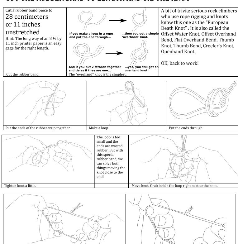
You can get more winds --and therefore more power--if you rub a small amount of baby shampoo (or even some liquid soap) into the rubber band after tying. Do NOT use oil, grease or any petroleum product on the rubber band—it will destroy it. While you're at it, add a drop to the propeller bearing/beads. Store the rubber in a dry place, away from direct light. More about Dragonfly Helicopters at sciencetoymaker.org.
